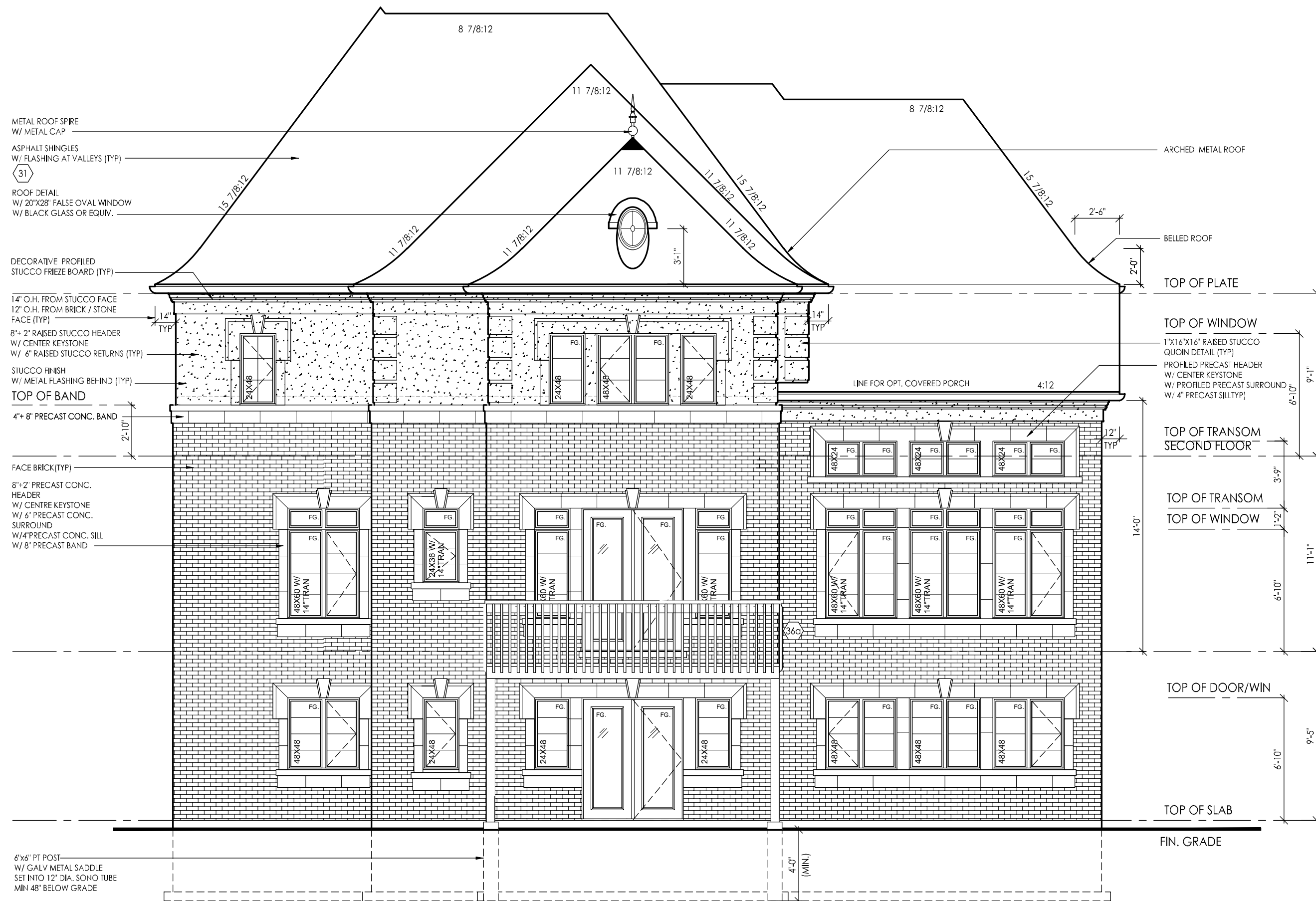
REAR ELEVATION 'C' - WOB CONDITION
