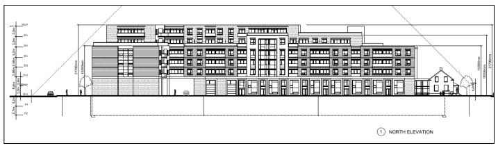
Figure 11: North Elevation of Proposed Development (HCA Architecture, 2023)
